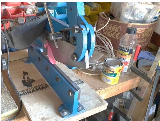
The Hafco Handshear from Machinery House in Manukau cuts through 5mm steel.
