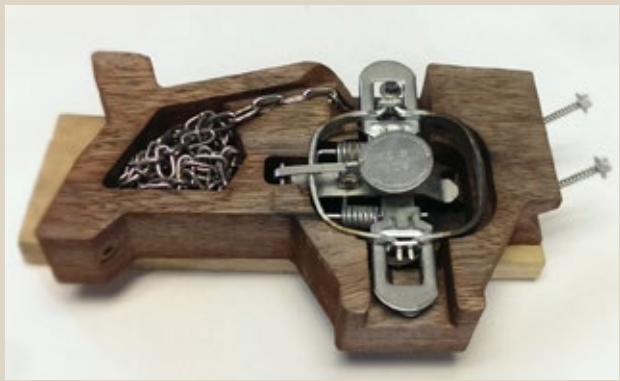
Sketch and photograph of prototype platform for automated possum leg hold trap system.
